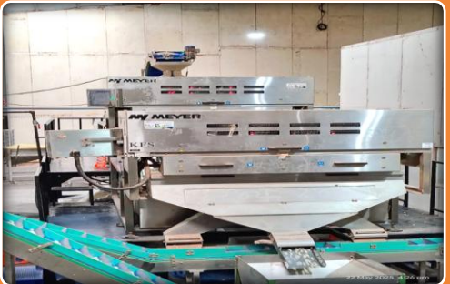
2-tonnes capacity color sorter for peeled cashew kernels
