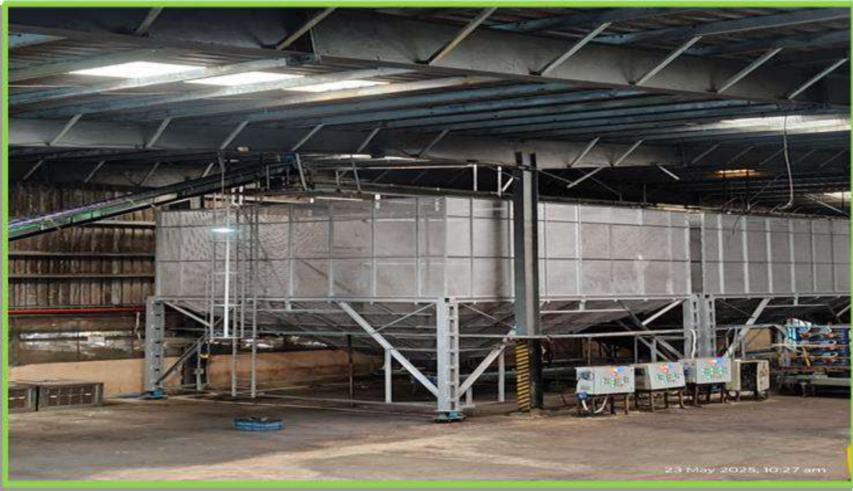
Silos for holding, drying, and batch-wise weighing of RCN
